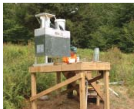
Michael McHale of the U.S. Geological Survey completes the installation of the mercury sampler in the Catskills. PHOTO: MARK WATSON.
